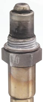
Thick carbon deposits on protective pipe
