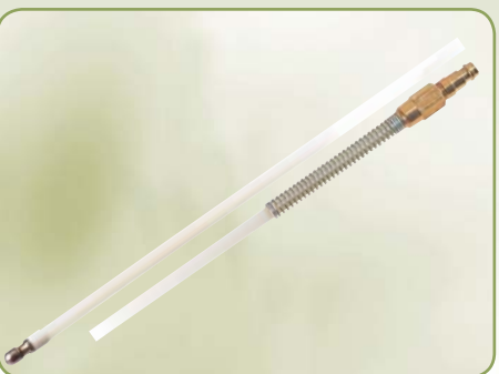
Teroson Flexible Nylon Probe The probe is used for spraying cavity protection materials into vehicle body cavities. It is suitable for curved and narrow cavities, which may also be very long. Teroson Hook Probe The probe is used for spraying cavity protection materials into vehicle body cavities, which are difficult to reach. For example: the 4 mm hook can be inserted through the drain holes in the bottom of a car door.
