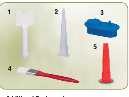
Additional Equipment 1 Door Skin Bead Nozzle, for use with Terostat 9100 (1K PUR). 2 Standard 310 ml nozzle, can be used with all 310 ml cartridges. 3 Cartridge Opener, for easy removal of seals on both ends of 310 ml cartridges. 4 Terolan brush, for use with Terolan Special 5 Direct Glazing Nozzle (Ter 20)
