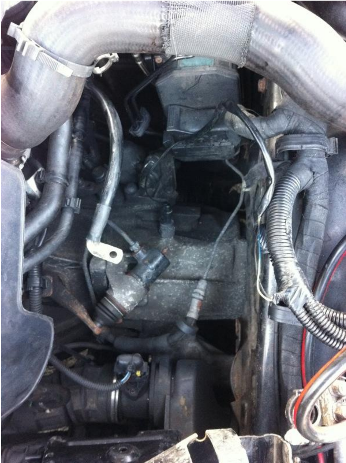
Step 3: taking apart the gear selector plate, clean, grease, replace bushes
