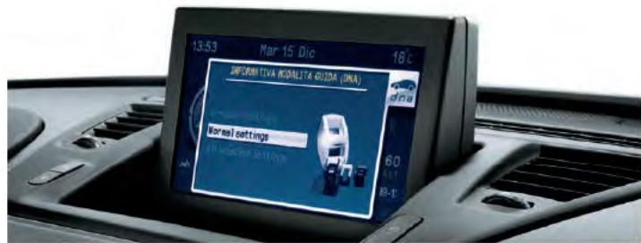
Alfa Romeo D.N.A. communicates with Radio NAV. The selected driving mode is conveniently shown on a pop-up display.
