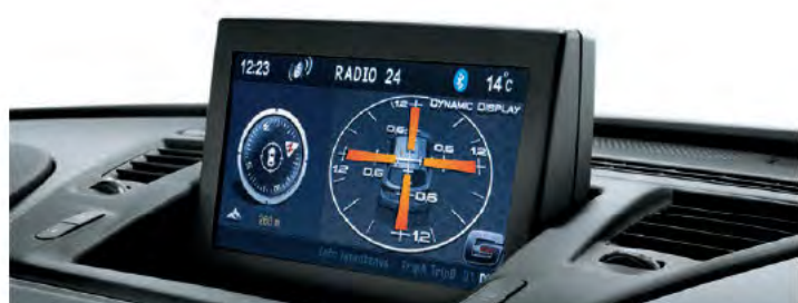
Radio NAV also shows the acceleration value (longitudinal and lateral) the car is subject to. (G-Force meter).
